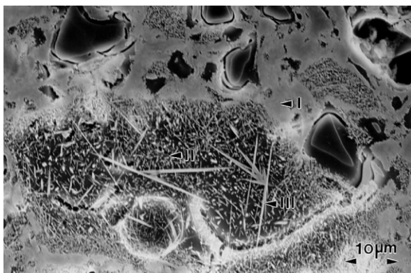
Fig. 2. Secondary electron SEM image of Wedgwood porcelain showing the 3 types of mullite.
